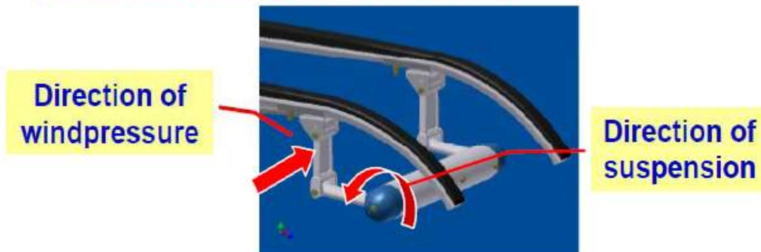
Aerodynamic influence to pan head suspension is eliminated by separation of wind pressure direction and working direction of suspension
